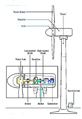
• **rotor blades** - capture wind's energy and convert it to rotational energy of shaft
